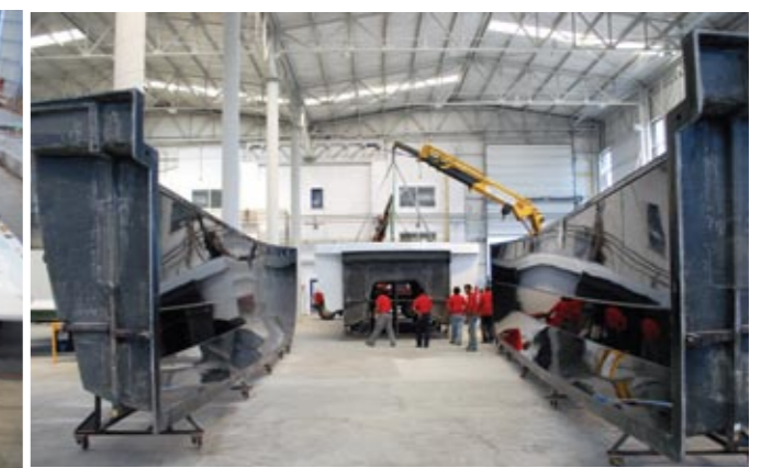
Labranda hull mold after demolding.
