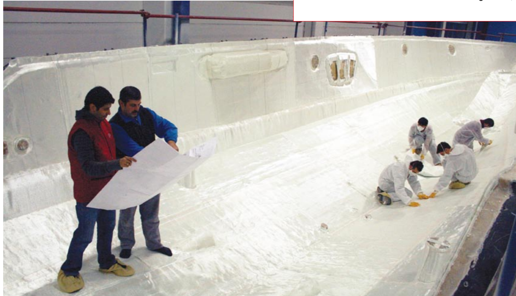
55 foot hull infusion preparation
