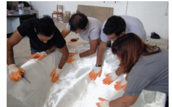
Fabric placement on mold
