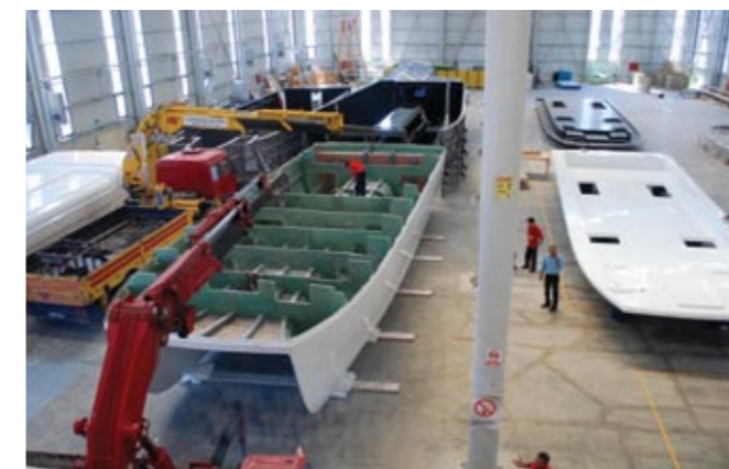
Labranda hull being demolded. Built exclusively by BGMS.
